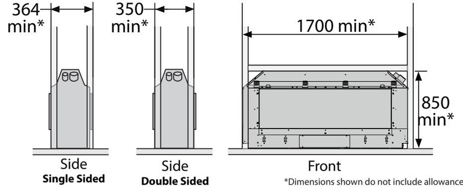
\*Dimensions shown do not include allowances for clearance to combustibles to the flue
