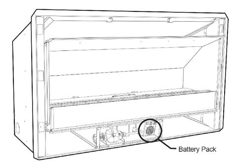
Remove the cap of the battery pack, turn it anti-clockwise until it stops, then pull. The batteries inside should slide out.
