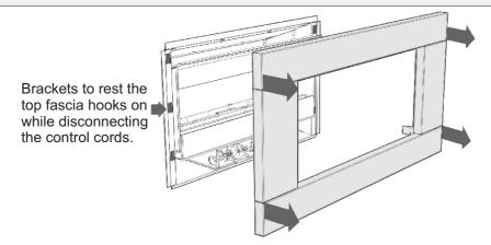
Reverse these steps to re-fit the Fascia, ensuring the two connections are correctly plugged in by testing the fire.
