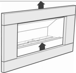
Now pull the fascia towards you, and rest the Fascia on the brackets half way down the firebox, or on the ground while you unplug the two cords connecting the fascia to the fire.
