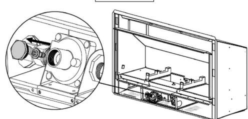
The pictures on the right show how the plunger should be orientated when re-inserted into the regulator.
