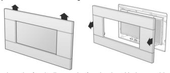
To replace the fascia, line up the four hooks with the matching receptacles on the fireplace and push the fascia into place and let it drop down, the fascia should now be securely in position.
