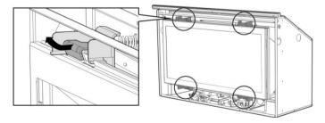
Do not operate the appliance if the glass has been broken, damaged, or the glass is not properly positioned/hooked onto the appliance.
