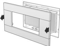
To replace the fascia, line up the four hooks with the matching receptacles on the fire and push the fascia into place and let it drop down, the fascia should now be securely in position
