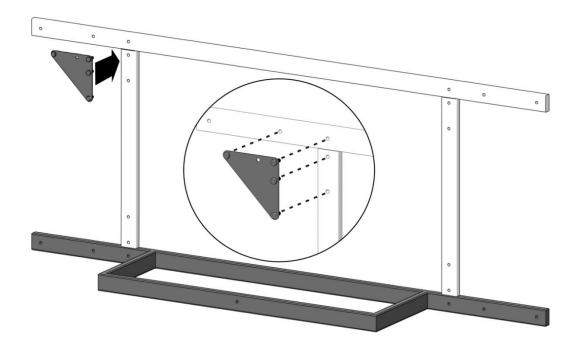
Attach the four triangle gussets to the Horizontal, Vertical and Middle sections as shown. Section Two is now complete.
