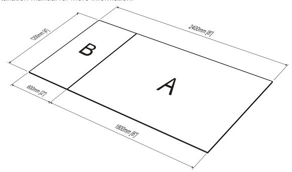
The second sheet should be cut into three pieces as illustrated below:
