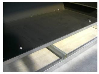
**Note:** when determining the position of the 6 mm holes, make sure the screws will not be in the way of the ash-pan. If the screws are positioned between 50 and 150 mm from the inside walls of the fire, they will clear the ash pan.
