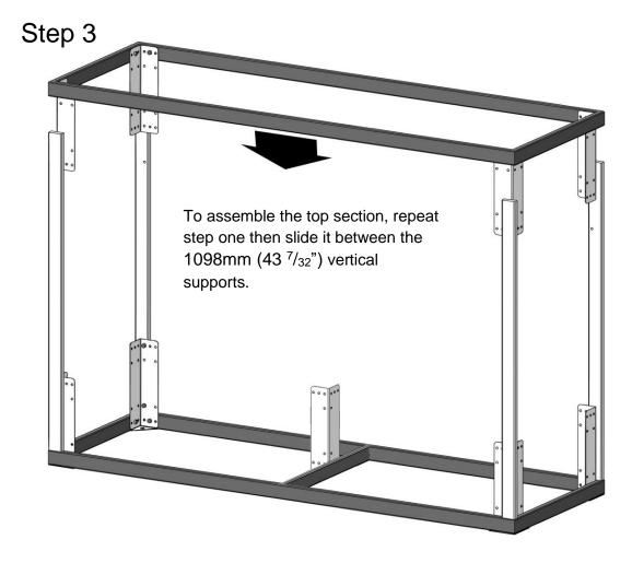
Once the top section is in place it can be attached with the hex bolts to the 1098mm (43  $^{7}/_{32}$ ") vertical supports. Section One is now complete.
