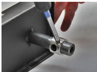
ULPG/Propane 11mm hole exposed
