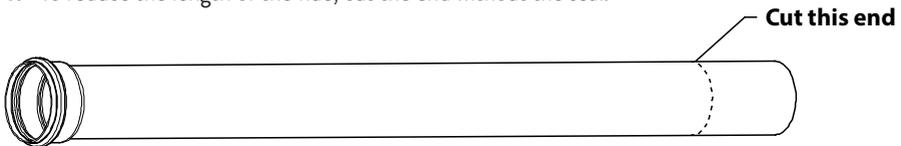
2. Ensure that any cut edges are completely de-burred and file a slightly bevel lead-in on the outer edge – failure to do so may damage the inner seal and create a leak path.
