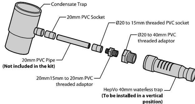
The above components (with the exception of the Ø20mm pipe) are included in the Escea Poly Pro starter kit. You will also need PVC cement and, depending on the particular install, Ø20mm elbows. This will allow the waterless trap to be connected to the Ø100mm condensate trap in a vertical position.
