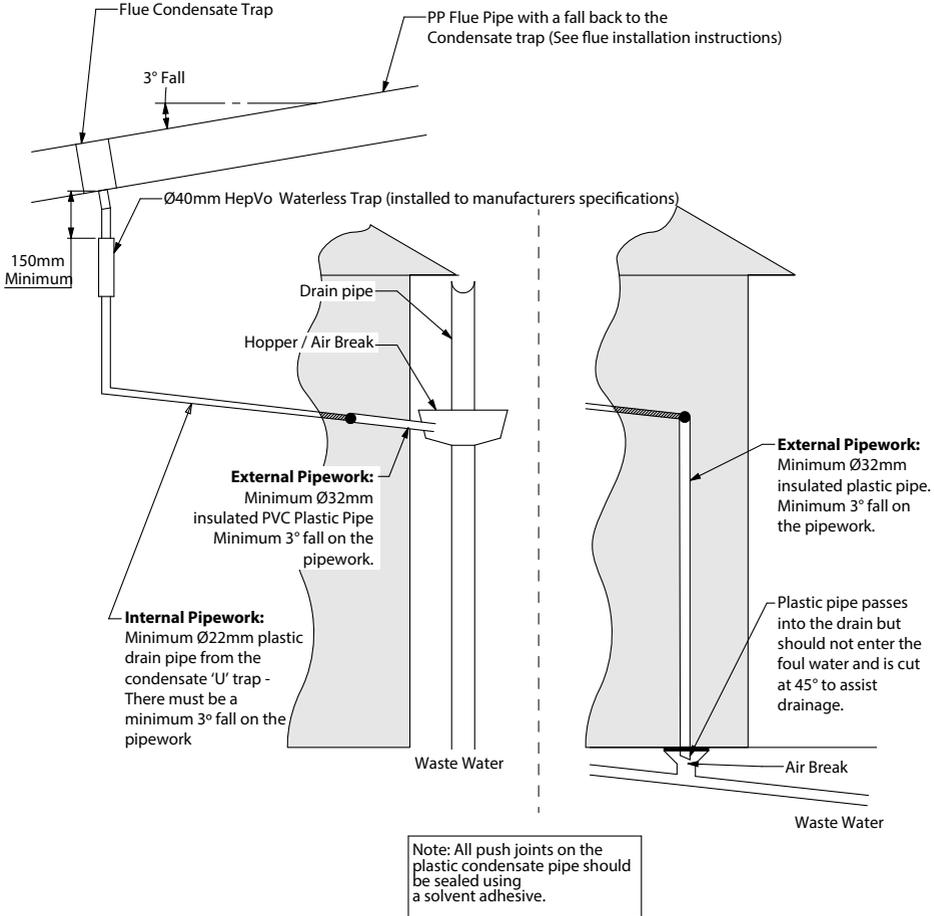
The use of an externally-run condensate drainage pipe, terminating at a suitable foul water discharge point or purpose-designed soak-away is acceptable, however, if this termination method is chosen, then the following measures should be adopted.
