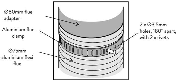
Step 2: Drill 2 x  $\text{\O}3.5\text{mm}$  holes,  $180^\circ$  apart, through the flue clamp, flexi flue, and flue adaptor. Secure the adaptor in place with two long rivets through the drilled holes, as shown in the diagram to the left.
