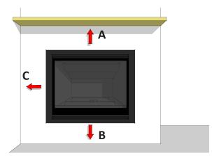
**Clearance Guidelines:** Adhere to combustible building material clearances in all directions around the fireplace: front clearance **1000mm.**
