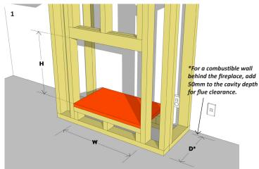
Build the chimney framework to meet the minimum fireplace opening requirements: 695mm W x 600mm H x 400mm D\*. Provide a 30mm thick base to allow for the fascia overhang below the fireplace.
