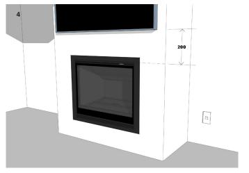
Install the appliance into the preformed cavity opening, fitting the flue spigot and connections as you go. Ensure the fireplace finishes over the wall lining. Fit the fascia. Complete the project by adding additional finishes or fixtures.
