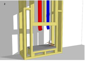
Prepare electrical, network connections, and gas supply. Run the flue pipes through the chosen pathway to the flue terminal. Connect Powerflue electrical cable at both ends.
