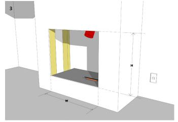
Attach wall linings to the framework, following the provided wall lining cutout dimensions: **695mm W x 560mm H**. Fit the spigot plate to the flue pipes.
