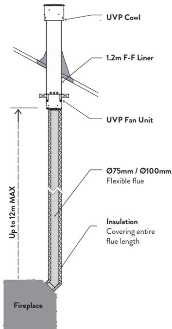
**Vertically Terminated:** utilises the Escea vertical power flue enclosure kit.
