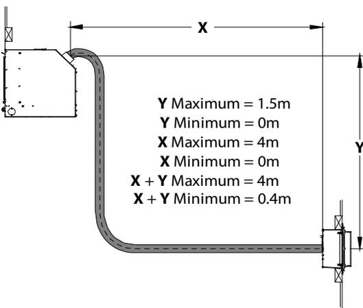
**Horizontally Terminated Downwards Flueing:** utilises the Escea horizontal power flue enclosure kit
