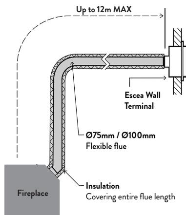
**Horizontally Terminated:** utilises the Escea horizontal power flue enclosure kit
