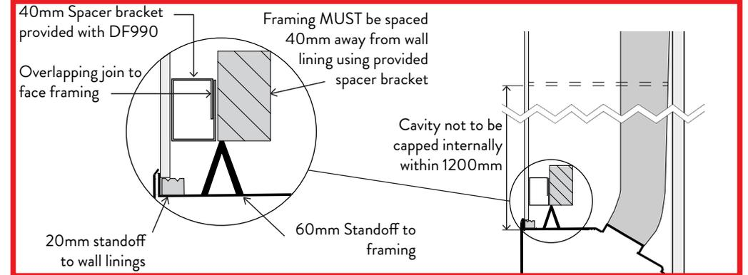
**\*WARNING:** The top standoffs must be adjusted to the upright position before the fireplace installation. All standoffs must remain in place for fireplace installation.
