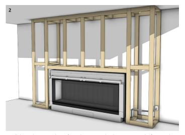
Install the appliance into the preformed opening in the chase. Secure to the framework  $% \left\{ 1\right\} =\left\{ 1\right\} =\left\{$ using the supplied nailing flanges. The fireplace should be flush with the wood framing. Install the electrical connection and gas supply.
