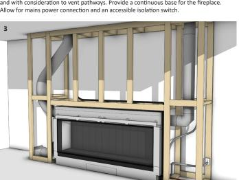
Connect the vent pipe to the fireplace and construct vent pathway to the vent termination. Connect Power-vent electrical supply from the fireplace to the vent termination. Install the heat duct system including the duct fan and duct fan electrical cable.
