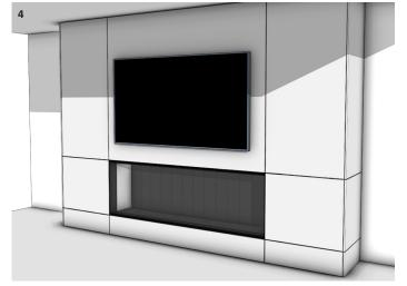
Fix the wall linings to the framework and the fireplace leaving a 1/4" gap to the glass opening. The wall lining can be bonded directly to the fireplace. Install any additional finishes or fixtures to complete the project.
