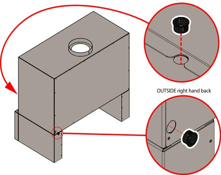
An alternative point of entry is down the flue pipe at the top. <u>Encase all wiring from the LE800 strain</u> relief to 1 metre beyond the last flue liner in 13mm split loom tube (not supplied).
