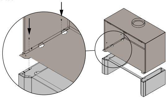
The electric cables can be run down through the "flue", up the right leg, or through the back of the freestanding console into the LE800 electric fire.
