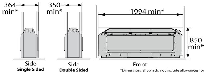
*\*Dimensions shown do not include allowances for clearance to combustibles to the flue*
