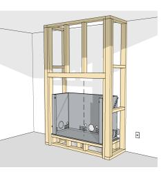
Install the structural base for the fireplace **40mm** behind the face of the timber framing.
