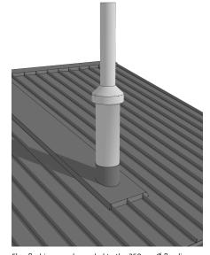
Flue flashings can be sealed to the 250mm Ø flue liner. The cone is sleeved over the 150mm Ø exhaust flue and sits on the spider bracket.
