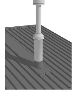
Anti-down draught cowl is fitted onto the 150mm Ø exhaust flue.
