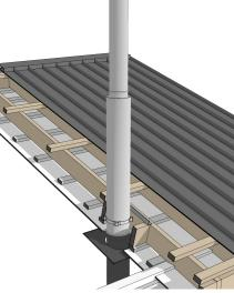
200mm Ø intake flue is fitted over the 150mm Ø exhaust flue from the fireplace to 915mm below the final 150mm Ø flue length. Ceiling plate should be fitted as this point.
