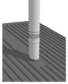
If using the designer flue shroud this is fitted over the standard flue kits, with the bottom shroud trimmed to within 100mm from the roof cladding.
