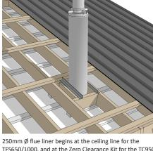
250mm Ø flue liner begins at the ceiling line for the TFS650/1000, and at the Zero Clearance Kit for the TC950. This fits over the 200mm Ø flue and extends to 915mm below the final 150mm Ø flue length. Flue spider is installed to the top of the intake and liner.
