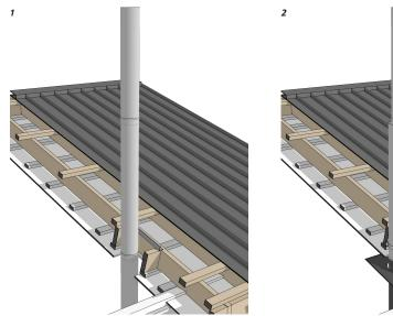
150mm Ø exhaust flue extends from the fireplace to the final cowl height. Spacer brackets are installed at regular intervals. Each length is installed crimp down and mechanically
