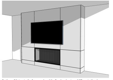
Fix the wall linings to the framework and the fireplace leaving a 1/4" gap to the glass opening. The wall lining can be bonded directly to the fireplace. vvInstall any additional finishes or fixtures to complete the project.
