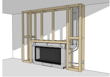
Install the electrical connection and gas supply. Connect the vent pipe to the fireplace and construct vent pathway to the vent termination. Connect Power-vent electrical supply from the fireplace to the vent termination.
