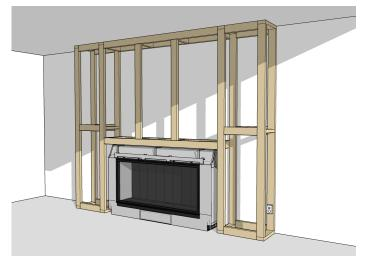
Install the appliance into the preformed opening in the chase. Secure to the framework using the supplied nailing flanges. The fireplace should be flush with the wood framing.
