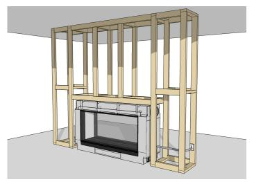
Install the appliance into the preformed opening in the chase. Secure to the framework using the supplied nailing flanges. The fireplace should be flush with the wood framing. Install the electrical connection and gas supply.
