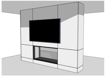
Fix the wall linings to the framework and the fireplace leaving a  $1/4^{\prime\prime}$  gap to the glass opening. The wall lining can be bonded directly to the fireplace. Install any additional finishes or fixtures to complete the project.
