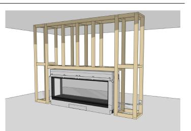
Install the appliance into the preformed opening in the chase. Secure to the framework using the supplied nailing flanges. The fireplace should be flush with the wood framing. Install the electrical connection and gas supply.
