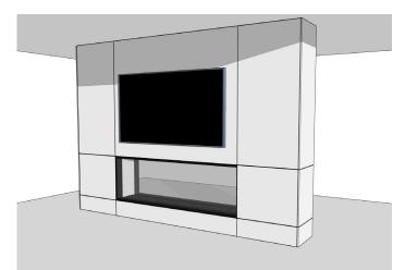
Fix the wall linings to the framework and the fireplace leaving a 1/4'' gap to the glass opening. The wall lining can be bonded directly to the fireplace. Install any additional finishes or fixtures to complete the project.
