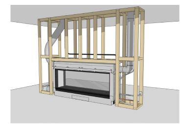
Connect the vent pipe to the fireplace and construct vent pathway to the vent termination. Connect Power-vent electrical supply from the fireplace to the vent termination. Install the heat duct system including the duct fan and duct fan electrical cable.
