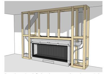
Connect the vent pipe to the fireplace and construct vent pathway to the vent termination. Connect Power-vent electrical supply from the fireplace to the vent termination. Install the heat duct system including the duct fan and duct fan electrical cable.
