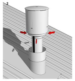
Install roof penetration flashing per local regulations. Attach 4"  $\times$  6 5/8" vent pipe to Power Vent Terminal. Connect Power Cable to fireplace, ensuring wiring by qualified electrician.
