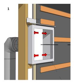
Establish the vent pipe centerline for the Horizontal Power Vent terminal, ensuring external clearances are met. Construct a 14 1/2" framework inside the wall, following minimum combustible clearance guidelines. Install the wall thimble into the wall to align with the siding.
