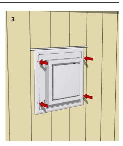
Install the Horizontal Power Vent Terminal onto the wall thimble, securely sealing and screwing it into place.
