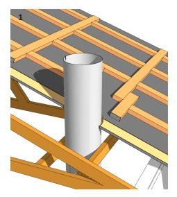
Locate and clear the vent pipe centerline. Create a 12" roof hole for the 11" vent liner, ensuring proper combustible material clearances and heights are met, as required.
