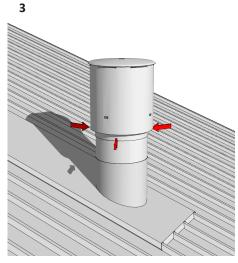
Fit the Vertical Power Vent Terminal onto the 11" Vent Liner and, seal and secure in place.
