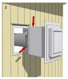
Attach the 4" x 6 5/8" vent pipe to the Vertical Power Vent Terminal. Connect the supplied power cable to the fireplace, with all wiring performed by a qualified electrician. Complete the wall siding installation, ensuring weathertightness in accordance with local building codes.
