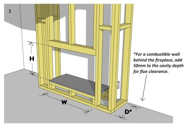
Build the chimney framework to meet the minimum fireplace opening requirements: 945mm W x 600mm H x 425mm D\*. Ensure a continuous base for the fireplace.
