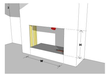
Attach wall linings to the framework, following the provided wall lining cutout dimensions:  $945mm\ W\ x\ 560mm\ H$ . Fit the spigot plate to the flue pipes.
