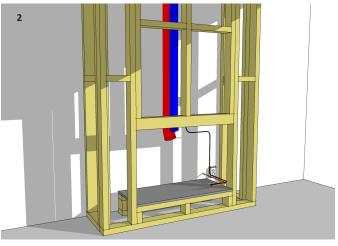
Prepare electrical, network connections, and gas supply. Run the flue pipes through the chosen pathway to the flue terminal. Connect Powerflue electrical cable at both ends.
