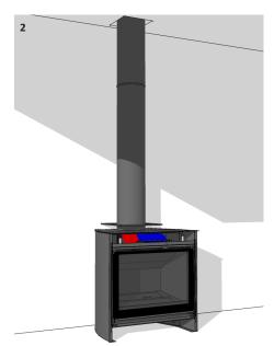
Secure the freestanding console to the floor. Install the DF700 fireplace into the freestanding console connecting the flue pipes, gas connections and powerflue electrical cable. Connect power supply to wall outlet. Complete commissioning of the fireplace and flue.
