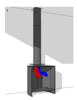
Locate the freestanding console in the desired location, complying with all clearances. Allow for an electrical outlet within 1m. Remove the upper and lower fascia from the console and set aside. Install the black rigid liners to the console, run the twin flexible flue pipes and powerflue
