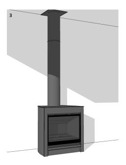
Fit the lower and upper fascia components back to the console. Install the ceiling plate to cover the hole for the flue pipes. Complete the project with any remaining fixtures and finishes.
