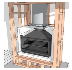
Select an appropriate location meeting all flue clearance and building requirements. Establish the flue centerline for obstruction-free installation. Build the framework, provide external ventilation, and install **AAC** panels as instructed. Secure the fireplace and the 250mm Ø flue, and temporarily position the Dropbox support bracket and flue Dropbox.
