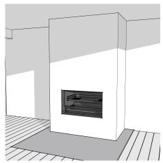
Fix a non-combustible substrate to the framework, detail the opening for wall lining protection from heat, and complete the installation with remaining fireplace components, wall finishes, and a floor protector/hearth.
