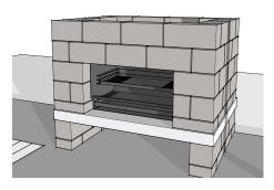
Provide exterior ventilation inlet hole either in the base or walls. Build the cavity to the required dimensions and finish option.
