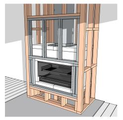
Finish the AAC Panel installation to enclose the heat cell. Conclude the flue installation by adding the remaining 350mm and 450mm Ø flue liners at the specified configuration and height. In this case, a lightweight steel frame is additionally employed on the front face to support the wall linings and finishes.
