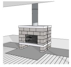
Install flue and spacer brackets, ensuring a 450mm clearance from the outer flue to combustible materials. Complete installation with remaining fireplace and flue components, and apply wall finishes and floor protector or hearth.
