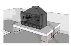
Select a location meeting all building and flue clearance requirements. Build a base to support the fireplace and/or cavity. Fix the fireplace into its final location. Restrain the fire to its base.
