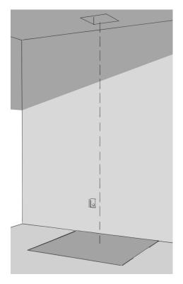
A location is selected with electrical supply within 1m of the fireplace. Obtain flue centreline to ensure the flue run is clear from obstructions. Install the floor protector, allowing for all requisite safety clearances.
