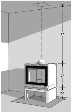
Install the fireplace on a plinth, base or preformed heat resistant structure following the TFS650 Installation Manual. Fix the fire to the plinth, base or structure and the plinth or base to the floor. It is recommended that only HHA approved/accredited tradespeople should be used to install this fireplace. \*See appliance dimensions over page.
