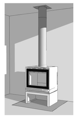
Install the flue and liner to the correct configuration and height. The ceiling plate should be fitted at this time. Complete the installation by installing any additional components. Operate the fireplace for the first week with a hot fire and the damper fully open.
