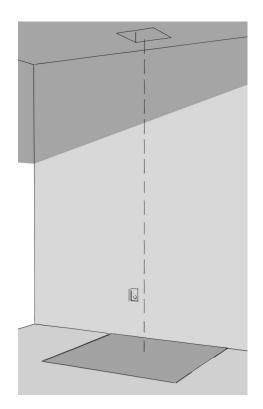
Select the desired location for the fireplace. Obtain flue centreline to ensure the flue run is clear from obstructions. Install the floor protector, allowing for all requisite safety clearances.
