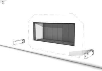
Attach wall linings to the framework and fireplace, maintaining the required gap from the fireplace trim or flange. Allow to cut out the wall lining around the PFS wall brackets. *Escea DS1150 Gas Fireplace shown*.
