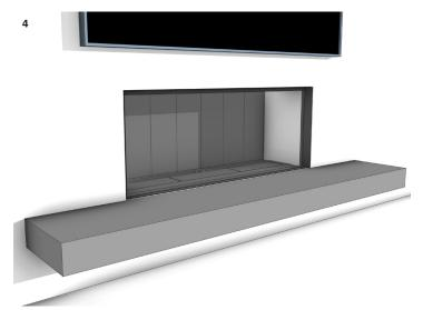
Complete the project by adding finishes to the hearth. Materials can be glue fixed with daubs of adhesive on the cross marks. Any material directly below an Escea Gas or Wood Fireplace must be non-combustible and heat resistant.
