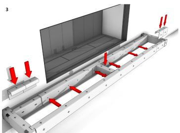
Install the PFS rails between the wall brackets, aligning the holes of the inner and outer telescopic rails. Rails slot into the wall brackets without fastenings. Secure each rail with at least 4x (M6 x 20) hex bolts and nuts. Attach the center bridge rail, bolting centrally using 4 x (M6 x 20) hex bolts and nuts. Use the provided packers on the inner rails for a flush finish; break off the needed amount and glue in place.
