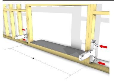
Construct the framework according to the minimum fireplace cavity and stud spacing requirements for PFS brackets. Attach the PFS wall brackets to the framework on each side of the fireplace, ensuring the vertical portions are flush with the framework's front. Secure the brackets to adjacent studs with the supplied 12G x 35mm Tek screws.
