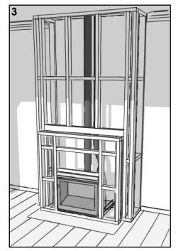
The fire is installed into the cavity and fixed to a continuous base.
