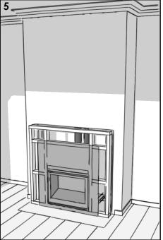
+ Wall linings are to finish behind the mantel. Ensure to accommodate this depth in framework calculations.
