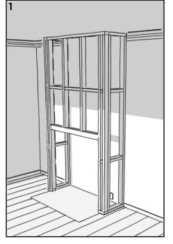
Standard building materials for construction of the chimney cavity.
