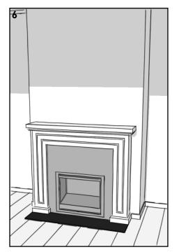
Mantel fixed to the framework through the sides, and holes filled.
