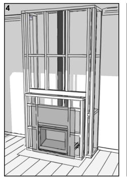
+ Infill panel is adhesive and/or screw fixed to the framing and the back face of the mantel.
