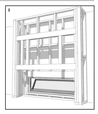
+ The cavity for the fire is created following the minimum requirements for the cavity, the flue and the duct components.
