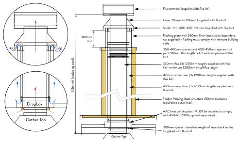
NOTE: The appliance & flue system shall be installed in accordance with AS/NZS 2918 and these specifications. NOTE: The flashing requirements must comply with the Installation Manual relevant section D3 on page 12 or E4 on page 21, depending on the installation method of choice.
