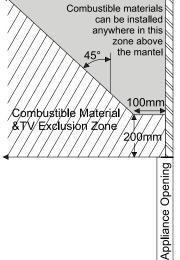
For DF700 & DF960 the minimum height for TV installation without a mantel installed: 200mm For DF990 a mantel is required
