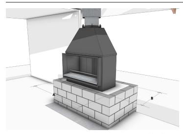
Cavity base is laid with fireplace base installed. **Fireplace weight: 127kg + Flue (40kg)** Initially, the fireplace is located towards the back of the cavity. Initial flue components can be installed.
