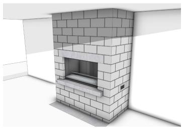
Detail the opening to cover the wall linings and protect from direct heat exposure. Complete the installation by installing the remaining fireplace components, apply any non-combustible finishes to the walls, and install the floor protector or hearth.
