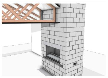
Complete the concrete structure to the prescribed height. The concrete cavity must extend at least above the roof line. Complete the flue installation by installing the remaining  $350/450 \text{mm} \ \emptyset$  flue and liners, and cowl.
