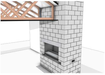
Complete the concrete structure to the prescribed height. The concrete cavity must extend at least above the roof line. Complete the flue installation by installing the remaining  $350/450 \text{mm} \ \emptyset$  flue and liners, and cowl.
