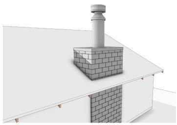
Fireplace is shifted forward into the cavity and final flue elements installed. Restrain the fire to its base structure. The flue height is a combination of the minimum flue length and the requirements of AS/NZS2918 External Clearances. Minimum flue length: 2.4m
