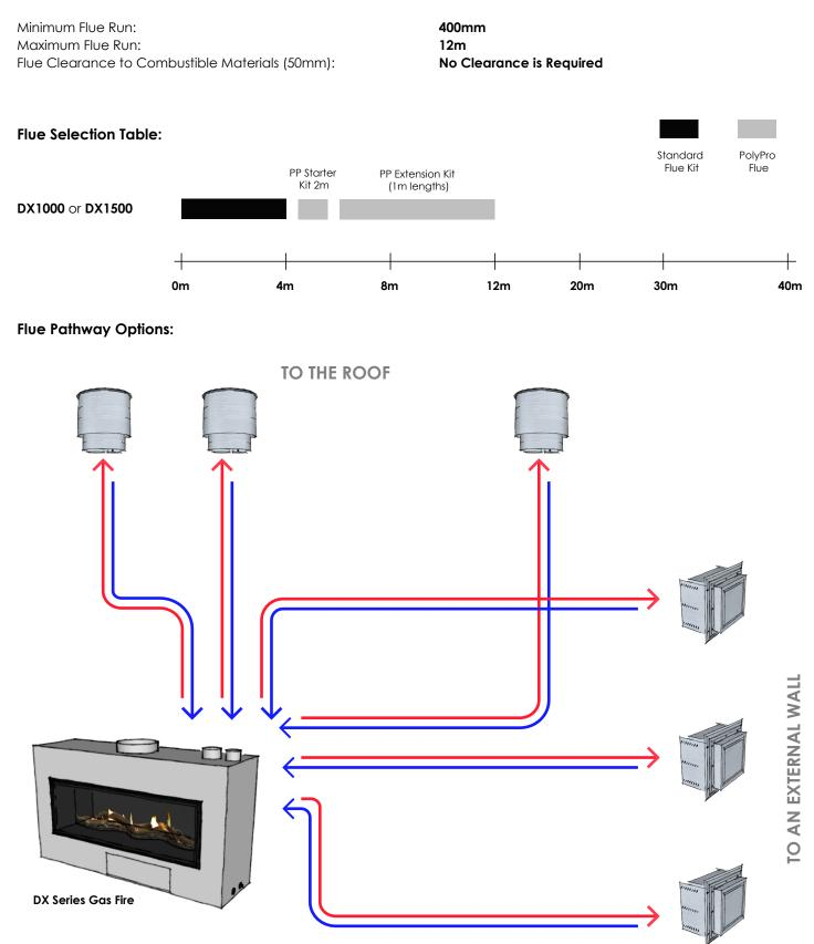
\* The installation and final location of the flue terminal must comply with the relevant **Escea Installation Instructions** and **AS/NZS5601 Gas Installations**. These provide guidance for clearances from the flue terminal to other elements of the building. Non-compliance to these clearances may decrease performance of the fire or flue, and/or pose a safety risk to the building users.
