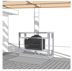
Fix the fireplace into its final location. Restrain the fire to the Kitset Enclosure. Install the flue and spacer brackets, ensuring a minimum clearance of **450mm** will be met from the 350mm flue to any adjacent combustible material.
