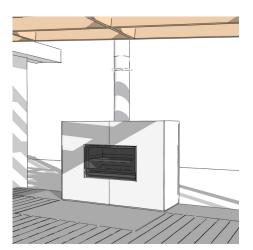
Fit the non-combustible substrate (where required) and prepare for finishing. Provide an inlet ventilation hole to the exterior. This is located on the back face in this instance.
