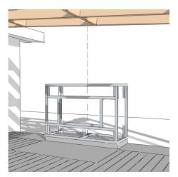
Build the EW5000 Kitset Enclosure following instructions supplied with the unit. Restrain the Kitset Enclosure to its base.
