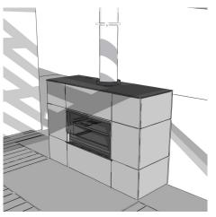
Complete the non-combustible finishes to the exterior carrying the ventilation hole through the finished cladding. Locate the chimney cap.
