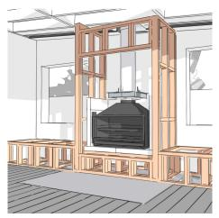
Install the rear, side and base AAC panels according to the manufacturers instructions. Fix the fireplace into the AAC heat cell alongside the 250mm Ø flue. Restrain the fire to its base. The Dropbox support bracket and flue Dropbox can be temporarily located.
