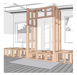
A location is selected meeting all requirements for flue clearances and the adjacent building. Obtain flue centreline to ensure the flue run is clear from obstructions. Build the framework to the required dimensions and provide the ventilation inlet hole to the exterior.
