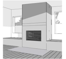
Fix the non-combustible substrate to the framework. Detail the opening to cover the wall linings and protect from direct heat exposure.
