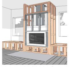
In this scenario an additional lightweight steel frame is used on the front face to support the wall linings and finishes.
