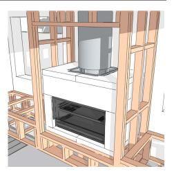
Finish the AAC Panel installation to close off the Heat cell. Complete the flue installation by installing the remaining 350mm and 450mm Ø flue liners to the correct configuration and height. Flue dropbox can be sealed in place.
