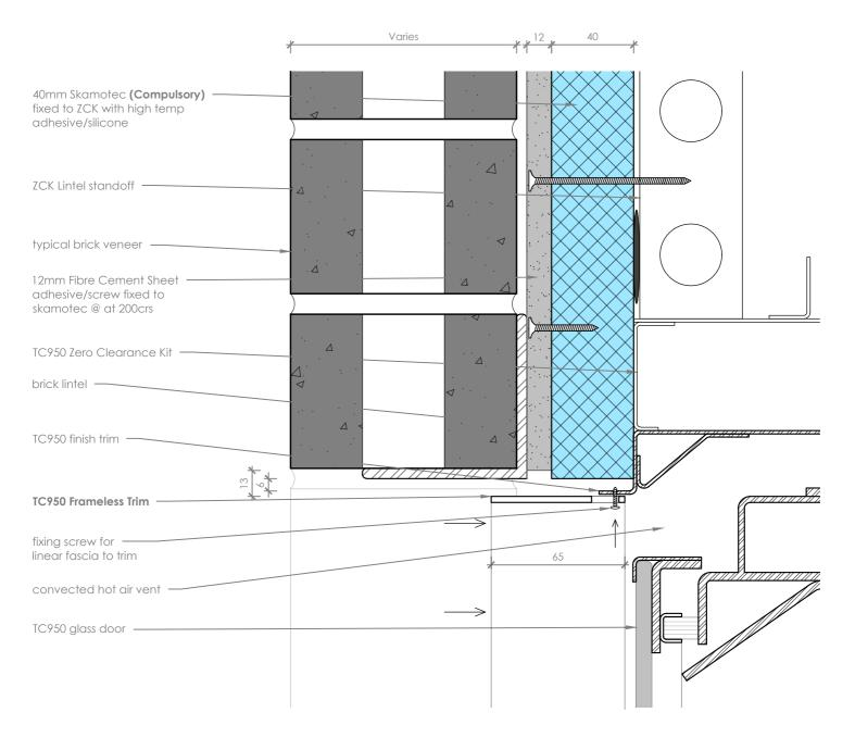
**TC950 Frameless Trim** is designed for deeper non-combustible finishes. The trim is designed to cover the junction of wall finish and substrate.
