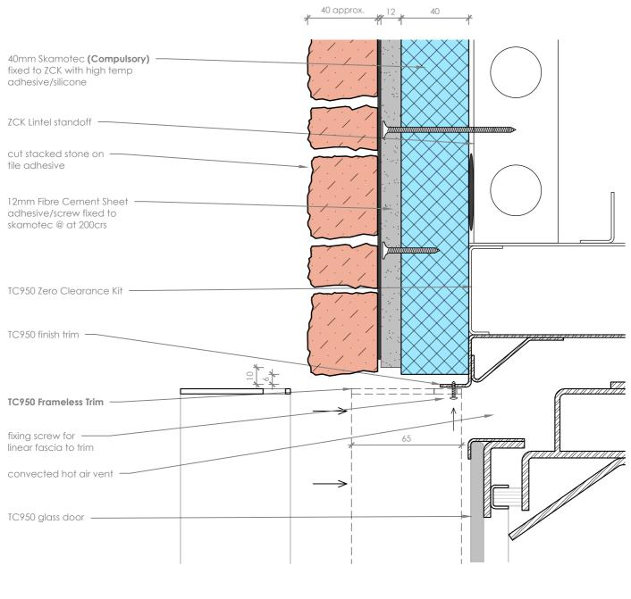
**TC950 Frameless Trim** is designed for deeper non-combustible finishes. The trim is designed to cover the junction of wall finish and substrate.
