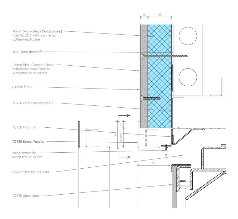
**TC950 Linear Fascia** is designed for paint, plaster or thin wall finishes. The fascia is designed to overlap the wall finish at the fireplace opening.
