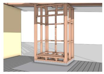
Obtain flue centreline to ensure the flue run is clear from obstructions. Build the framework to the required dimensions and provide the ventilation inlet hole to the exterior. Fireplace weight: 127kg + Flue (40kg)
