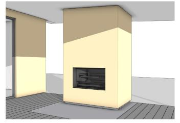
Detail the opening to cover the wall linings and protect from direct heat exposure. Complete the installation by installing the remaining fireplace components, apply any finishes to the walls, and install the floor protector or hearth.
