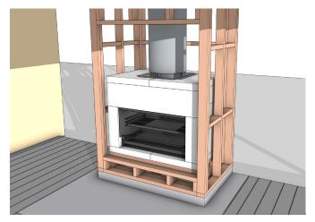
Install the EW5000 into the AAC panel cavity according to the manufacturers instructions. Connect dropbox and flue components. Restrain the fire to its base. Complete the flue installation by installing the remaining 350mm and 450mm  $\emptyset$  flue liners to the correct configuration and height.
