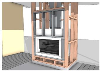
In this scenario an additional lightweight steel frame is used on the front face to support the wall linings and finishes.
