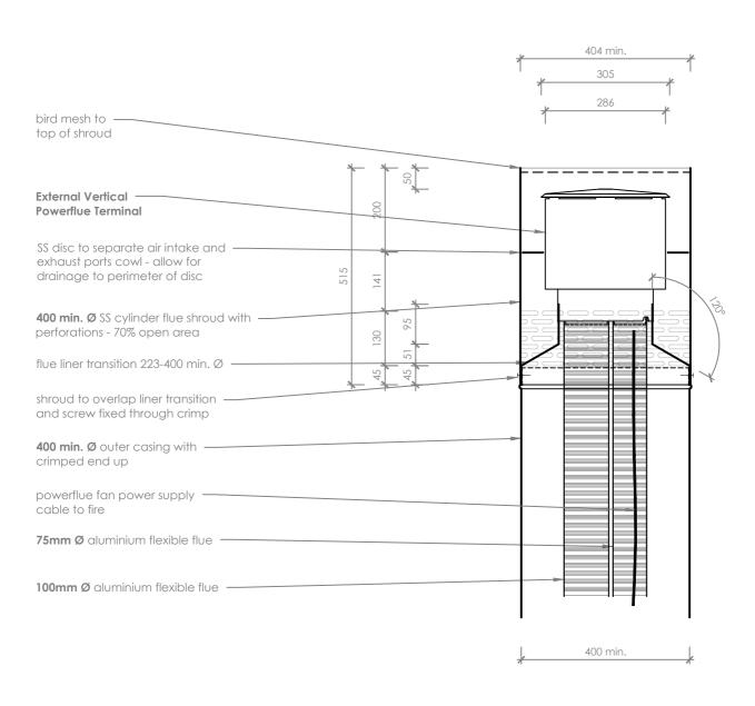
**Flue Detail** scale 1:10
