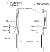
When building a recess the flueing must be considered. Shown right is the minimum distances possible when offsetting the flue to allow for a recess above.
