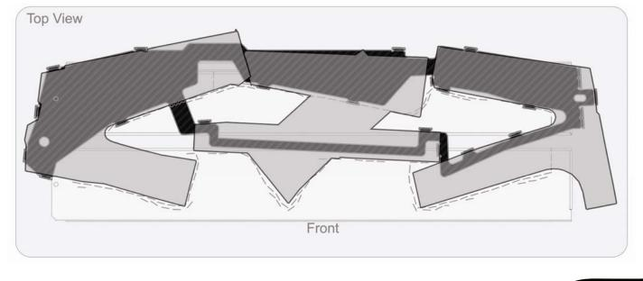
Note: The front right hand log will be raised slightly off the burners to improve airflow.
