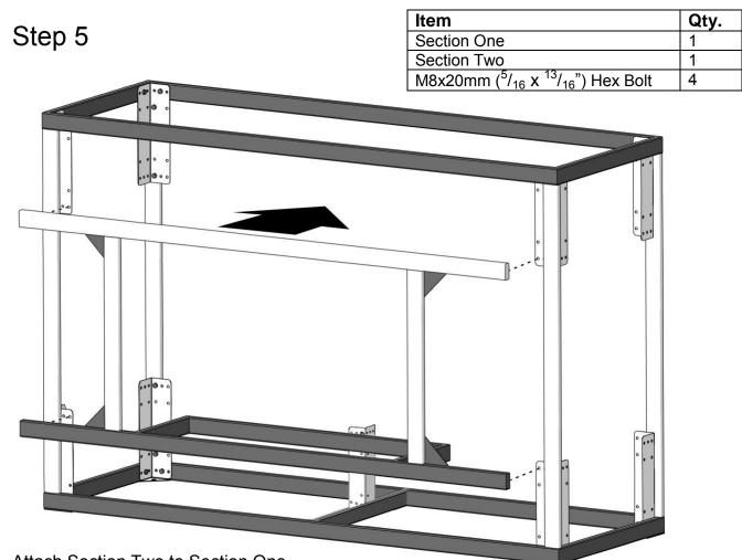
Attach Section Two to Section One.
