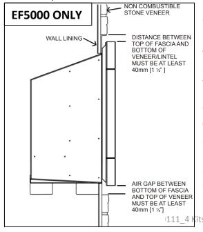
The unit was designed with 300mm (11  $^{13}/_{16}$ ") x 300mm (11  $^{13}/_{16}$ ") tiles in mind, but any finish from stone veneer, rough-cast plaster, timber or anything else that you can think of, could be used to good effect.
