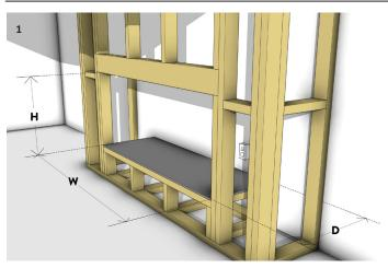
Build the chimney framework with consideration to the minimum cavity opening requirements described above for either the single or double niche. Ensure a continuous base for the fireplace. *Cavity for LE800 Electric Fireplace with single niche shown*.
