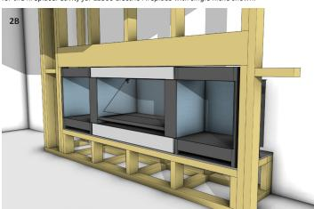
Install the LE Series Fireplace and niche following the instructions provided, connecting and confirming power supply to fireplace and niche. Both the LE Series Fireplace and Niche should be flush with the framework. *LE800 Electric Fireplace with double niche shown*.
