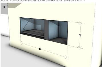
Attach wall linings to the framework and fireplace, maintaining a 3mm gap from the fireplace trim. Follow the provided wall lining cutout dimensions above. Complete the project by adding an additional LE Series Linear Trim or other fixtures and finishes.
