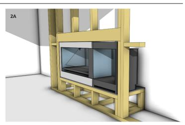
Install the LE Series Fireplace and niche following the instructions provided, connecting and confirming power supply to fireplace and niche. Both the LE Series Fireplace and Niche should be flush with the framework. *LE800 Electric Fireplace with single niche shown*.
