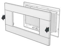
To replace the fascia, line up the four hooks with the matching receptacles on the fire and push the fascia into place and let it drop down, the fascia should now be securely in position
