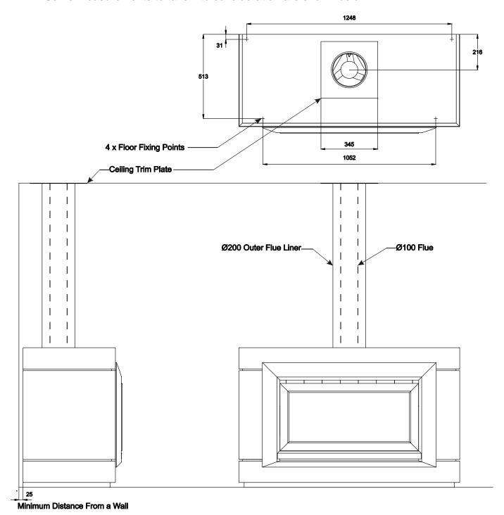
Note: Sealing around the hole in the ceiling and flue terminal is the responsibility of the installer and should be completed in accordance with local regulations The flue should be connected to the fire in accordance with local regulations based on the following illustration
