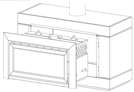
The Free Standing Unit should be assembled and fixed to the floor before the installation of the Outer Skin Kit. Ensure that gas and electricity services to the gas appliance have been taken into account before finalising the Free Standing Unit position.
