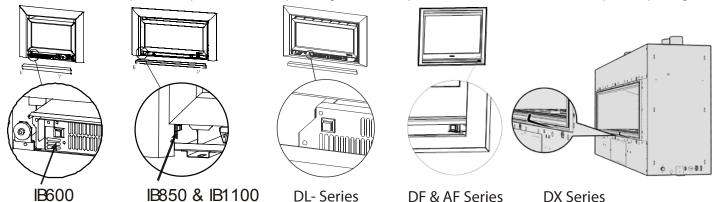
Note: you will need a long thin tool (such as an allen key) and insert this through the opening on an angle as shown.
