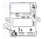
In order to do this, you must turn the lock/unlock switch on the fireplace control unit box (A) to the UNLOCK position.
