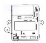
In order to do this, you must turn the lock/unlock switch on the fireplace control unit box (A) to the UNLOCK position.
